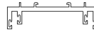
9160 2 9/16" Deep Adjustable Side Lite Base Horiz. W/ BRK. MTL. Use W/9161 Vertical Use (2) 9133 Glass Stops Use W104 Weathering
