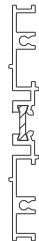
1G14 Adjustable Side Lite Base Vertical W/ BRK. MTL. Use W/ 1G13
