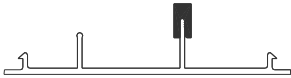
K318 3" Perimeter Adaptor Clip Pkg. Use Only W/ 9247 at Head / Sill ( See 9246 & FS93 )
