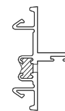
4441 5/8" Snap In Door Stop Used at Door Headers Only. Used W/2" Door
