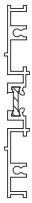
1G14 4 1/2" Deep Adjustable Side Lite Base Vertical W/BRK. MTL. Use W/1G13 Horizontal
