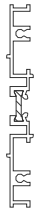
1G14 4 ½" Deep Adjustable Side Lite Base Vertical Mullion W/BRK. MTL. Use W/1G13 Horiz.
