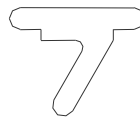
W104 Weather Seal Gasket Use W/ Expansion Mulls, @ Variable Mulls, or Adj. Height Side Lite Bases
