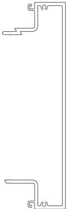
9231 8" Horizontal Self-Mating Use (2) K129 Shear Block Use Removable Stop Horizontals Above & Below
